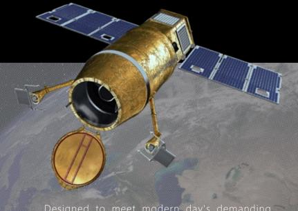
Designed to meet modern day's demanding operational challenges ,the EROS NG Constellation is comprised out of 3 proven and mature platforms providing 30cm resolution Ultra-Sharp imagery
